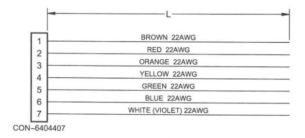
NOTE: FOR CABLES LONGER THAN 4 FT.(48in.), USE CBL-22AWG-8COND-SH.
